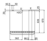
E: Electric connection D: Drain for water H2O: Water inlet 3/4"
