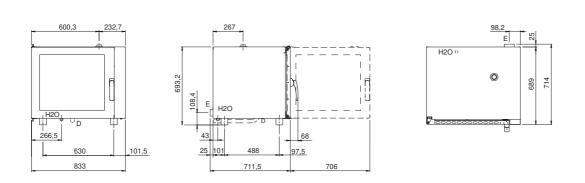
E: Electric connection D: Drain for water H2O: Water inlet 3/4"
