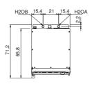
E: Electric connection D: Drain for water H2OA: Water inlet
